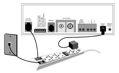
5. Plug in your standard, single line telephone to the "PROGRAM PHONE" jack on the front of your FreezeAlarm. See Figure below.
